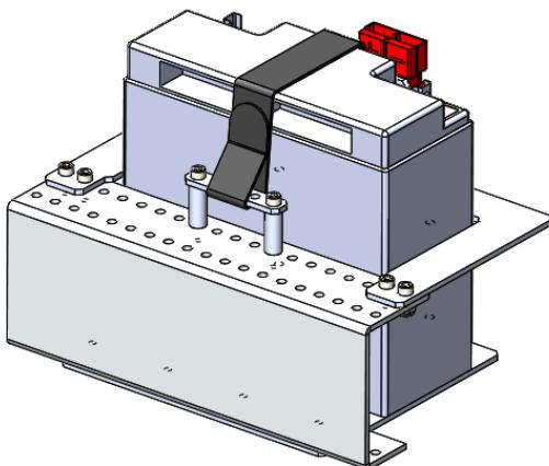
**Note:** Battery wires and connector half not shown.
