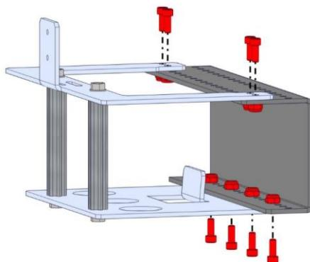
**Step 5:** Secure the Robot Side SB-Series Battery Connector (not included) to the tab on the C Plate using two #6-32 x 0.750" Hex Head Screws (am-1564) and #6-32 Nylock Jam Nuts (am-1419). The wires from this connector should go to your main robot breaker and power distribution panel.
