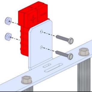
**Note:** The screws should be oriented such that the heads of the screws are on the Tab side.
