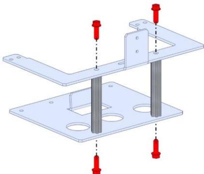
**Step 2:** Slide the assembly over the End Plate. The C Plate and Bottom Plate should be installed on the top and bottom of the flanges on the End Plate, respectively.
