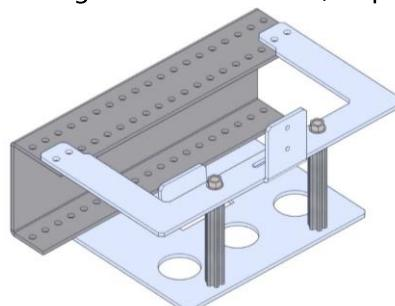
**Note:** The assembly may need to be slightly flexed to fit over the flanges on the End Plate.
